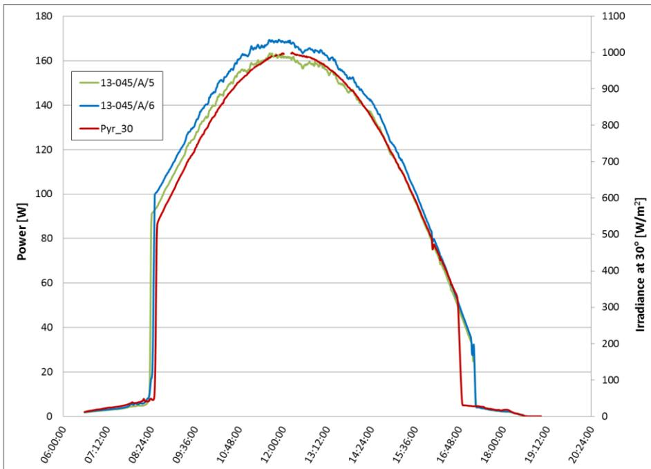
**Figure 8:** Power [W] for the 13-045/A/5/noRefl and 13-045/A/6/Refl modules and irradiance at 30° [W/m<sup>2</sup>] on the 13.09.2013.
