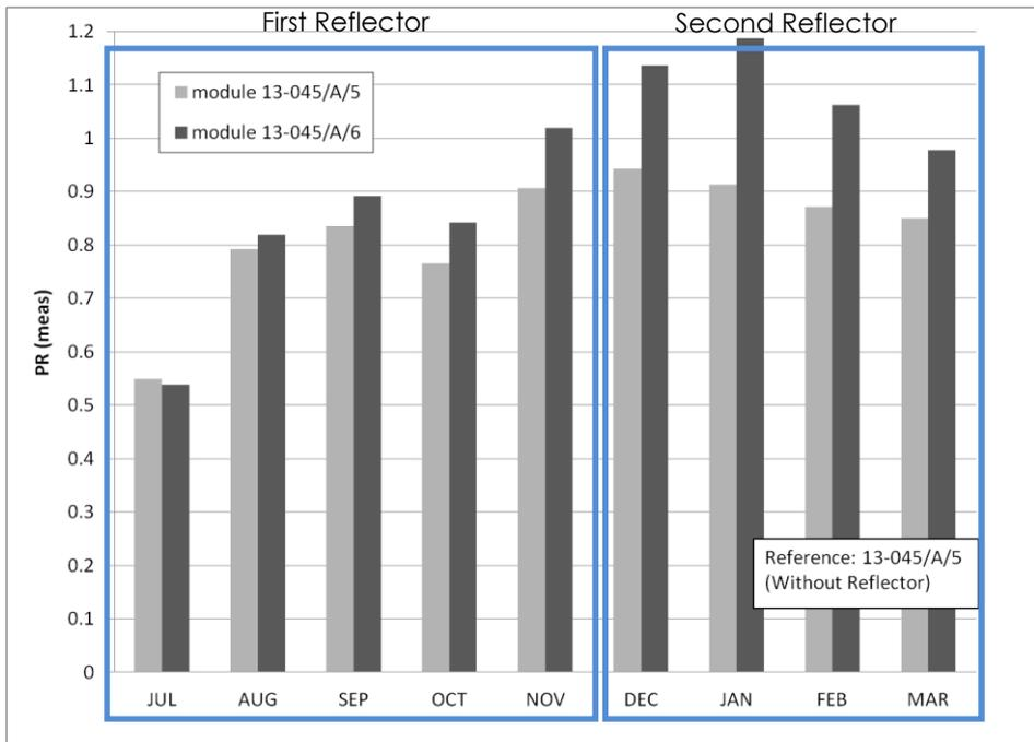
Figure 5: Performance Ratio comparison of the two modules between July 2013 and March 2014.
