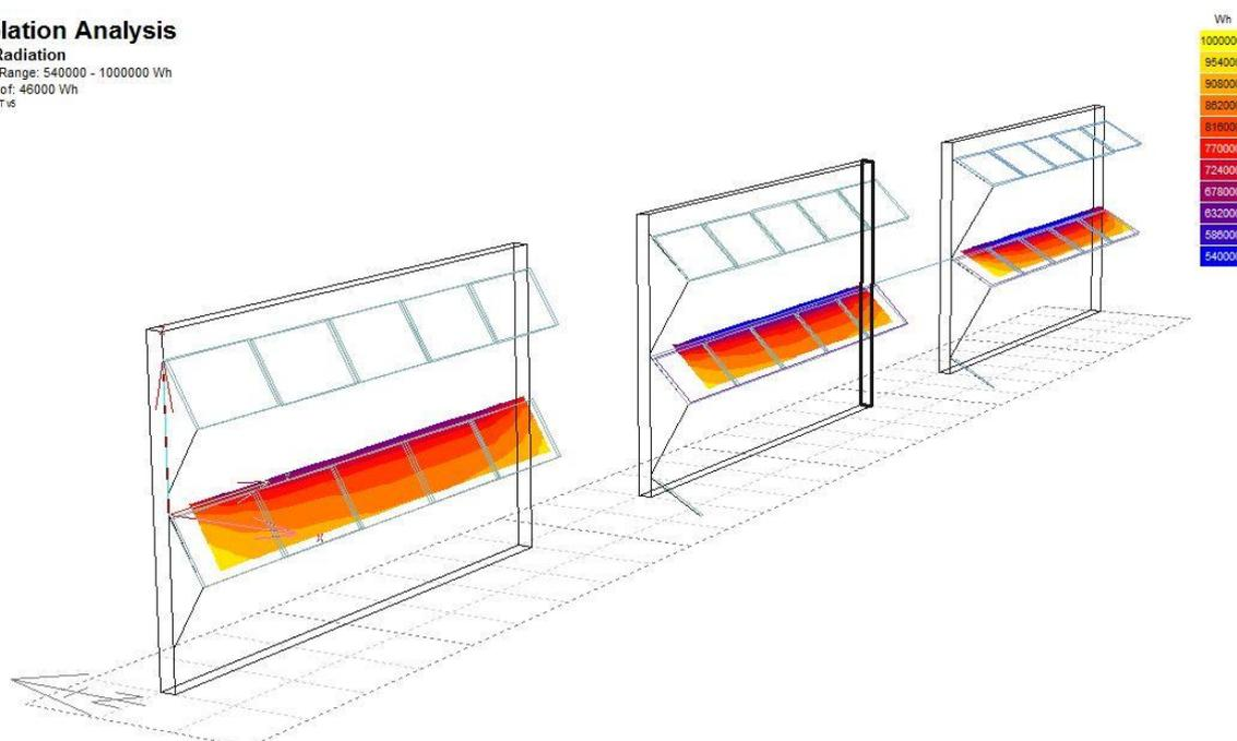
**Figura 16:** The picture shows the insolation on the PV modules with three different configurations: from the left situation the modules are tilted respectively of about 60°, 45° and 30°.
