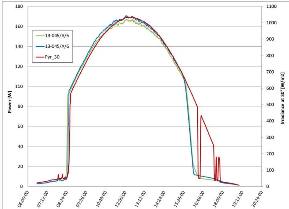
**Figure 7:** Power [W] for the 13-045/A/5/noRefl and 13-045/A/6/Refl modules and irradiance at 30° [W/m<sup>2</sup>] on the 20.08.2013.
