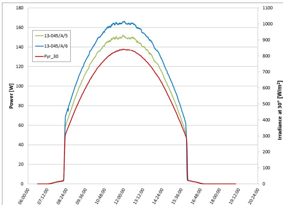
**Figure 10:** Power [W] for the 13-045/A/5/noRefl and 13-045/A/6/Refl modules and irradiance at 30° [W/m<sup>2</sup>] on the 11.11.2013.
