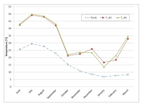
**Figure 13:** Monthly average ambient temperature (Ta) and monthly average temperature at the back of the two modules (13-045/A/5/noRefl and 13-045/A/6/Refl).
