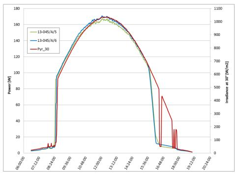
Figure 7: Power [W] for the 13-045/A/5/noRefl and 13-045/A/6/Refl modules and irradiance at  $30^{\circ}$  [W/m<sup>2</sup>] on the 20.08.2013.
