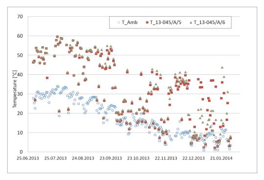
Figure 14: Daily average ambient temperature (Ta) and daily average temperature at the back of the two modules (13-045/A/5/noRefl and 13-045/A/6/Refl).
