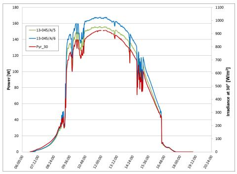
Figure 9: Power [W] for the 13-045/A/5/noRefl and 13-045/A/6/Refl modules on the 11.10.2013.
