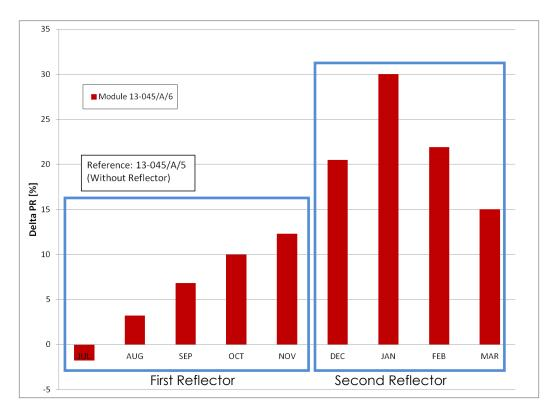
**Figure 11:** Aggregated results of the difference of PR between the two modules (13-045/A/5/noRefl and 13-045/A/6/Refl) for the whole monitoring period.
