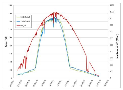
Figure 6: Power [W] for the 13-045/A/5/noRefl and 13-045/A/6/Refl modules and irradiance at 30° [W/m<sup>2</sup>] on the 15.07.2013.
