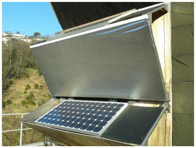
Figure 2: Second configuration. In December the first reflector was substituted by a new material. 13-045/A/5/noRefl module during the month of January
