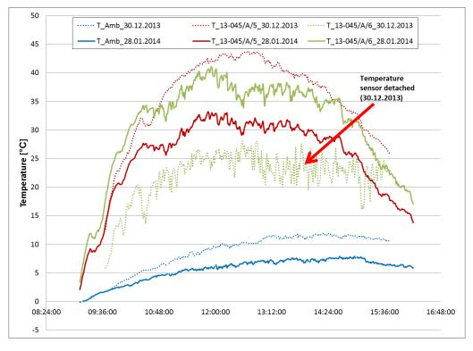
**Figure 15:** Minute values of ambient temperature (Ta) and minute values of temperature at the back of the two modules (13-045/A/5/noRefl and 13-045/A/6/Refl) for the 30.12.2013 (dotted lines, temperature sensor for A/6 detached) and 28.01.2014 (continuous lines).
