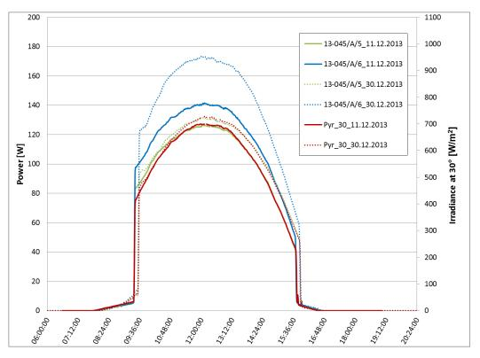
**Figure 12:** Power of the two modules (13-045/A/5/noRefl and 13-045/A/6/Refl) and irradiance at 30° on 11.12.2013 (before the new reflector mounting) and 30.12.2013 (after the new reflector mounting).
