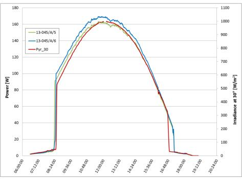
Figure 8: Power [W] for the 13-045/A/5/noRefl and 13-045/A/6/Refl modules and irradiance at  $30^{\circ}$  [W/m<sup>2</sup>] on the 13.09.2013.
