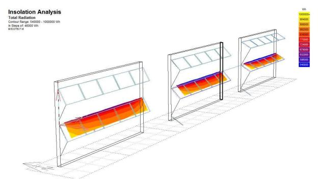
**Figura 16:** The picture shows the insolation on the PV modules with three different configurations: from the left situation the modules are tilted respectively of about 60°, 45° and 30°.
