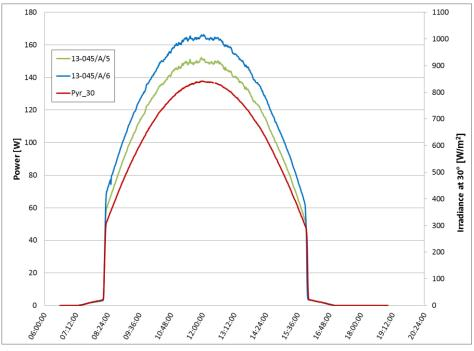
Figure 10: Power [W] for the 13-045/A/5/noRefl and 13-045/A/6/Refl modules and irradiance at  $30^{\circ}$  [W/m<sup>2</sup>] on the 11.11.2013.
